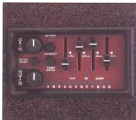
A: The new Optima preamp has a tunable notch filter and a built-in chromatic tuner.
