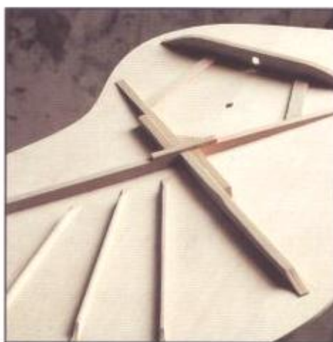
K: The highly developed "X" bracing pattern combines strength with exceptional freedom of vibration.
